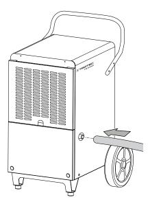
2. Guide the other hose end to a suitable drain or sufficiently dimensioned collection container. Please note that the hose must not be kinked.
