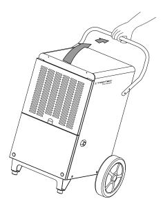
• Only wheel the device on a level and smooth surface.
