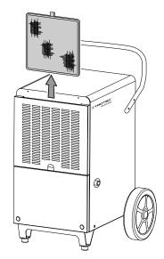
2. Clean the filter using a slightly damp, soft, lint-free cloth. If the filter is heavily contaminated, clean it with warm water mixed with a neutral cleaning agent.
