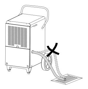
3. Make sure that the condensation drain hose is installed with a continuous decline.
